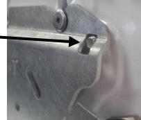
Unscrew the locking screw with Torx T8 tool, without removing the screw from the plate so as not to lose the seal.
