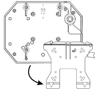
**Step 4:** Fix the four mountings bracket on the reader using the four-metal plate mounting screws.
