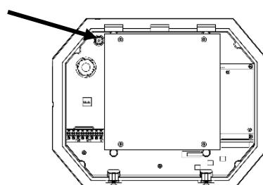
**Step 3:** Remove the metal mounting plate by exerting pressure on the metal plate while sliding it.
